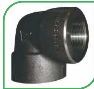
ELBOW 90 NPT/SW 2000/3000/6000 PSI Body: SS / Carbon Steel Size: 1/8" to 4"
